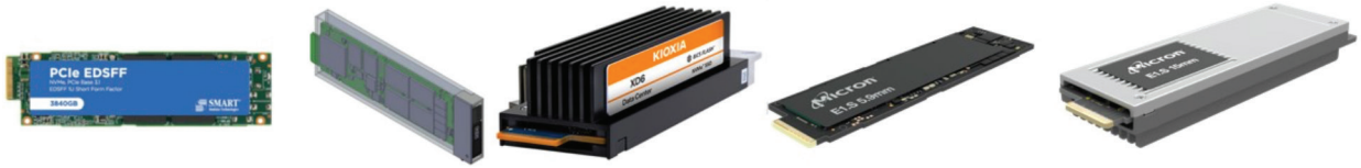
Figure 1: left to right: E1.S 5.9mm (courtesy of SMART Modular Systems); E1.S Symmetric Enclosure (courtesy of Intel); E1.S (courtesy of KIOXIA); E1.S 5.9mm (courtesy of Micron); E1.S 15mm (courtesy of Micron)
